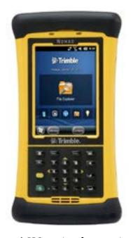
resolution color images in the field with their precise locations stored, and an integrated GPS receiver for mapping and navigation applications. It boasts an advanced Trimble GPS antenna design which reads the full constellation of satellite signals plus SBAS. It gives 2-4 meter positional accuracy, with GPS acquisition in seconds, and works under thick canopy, in canyons or near tall buildings; ideal for both rural and urban data collection requirements.
